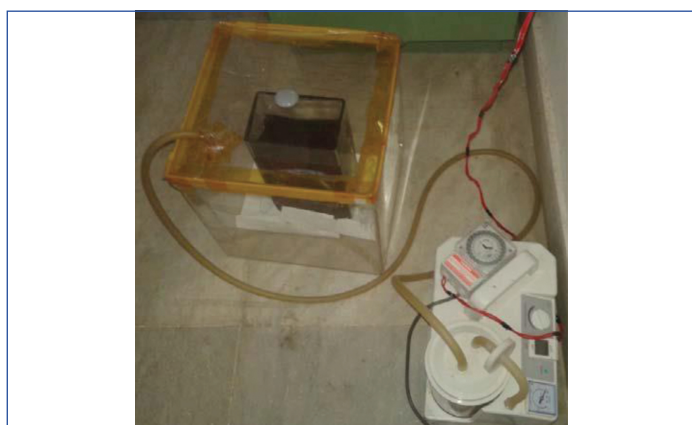
[Table/Fig-2]: Hoover chamber: impregnation with melamine.
